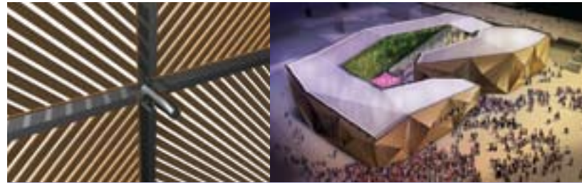
DETAIL OF STEEL SUPPORTING STRUCTURE FOR WRC CLADDING
