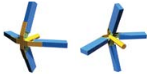
DETAIL OF STEEL SUPPORTING STRUCTURE FOR WRC CLADDING
